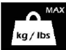
If the lift stops because of an overload (an attempt to lift more than the safe working load) the overload symbol will appear on the LCD display and the lift will cease. Lower the boom and remove excess weight.
