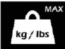
If the lift stops because of an overload (an attempt to lift more than the safe working load) the overload symbol will appear on the LCD display and the lift will cease. Lower the boom and remove excess weight.
