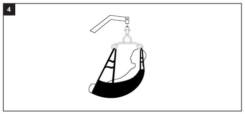
Raise the lift to the required height. NOTE: It may be necessary to support the head while the patient is suspended.
