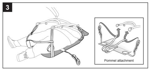
Move the lift into position above the client, keeping the cradle hooks away from the client's face. Attach the shoulder and leg straps to the respective front and rear hooks on the cradle, ensuring to feed each leg strap through the corresponding pommel loop (see diagram above). Adjust the head support to suit client comfort.
